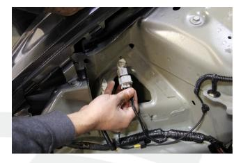
Figure 32 (Connector G012 location)
