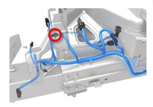
Figure 28 (Connector X261 location)
