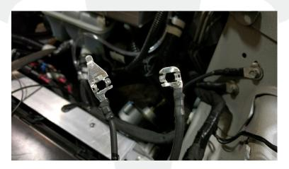
Figure 14 (LH and RH eyelets)
