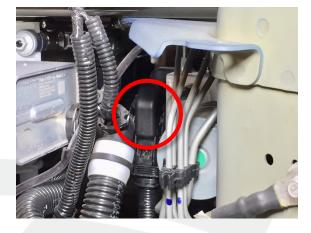
Figure 4 (Connector X151 location)
