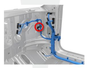
Figure 37 (Connector X172 and X121 locations)
