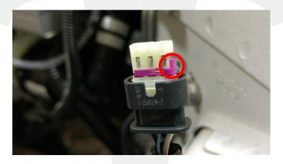
Figure 19 (Slide out to open, in to close)
