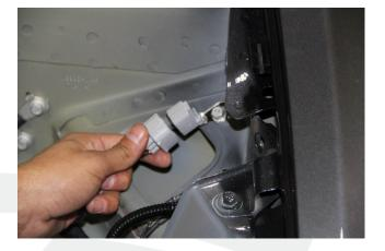
Figure 23 (Connector G011 location)
